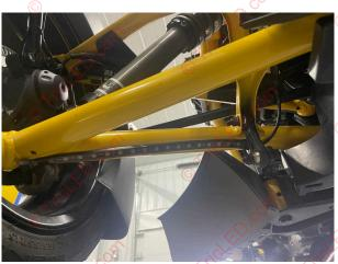
Test fit the LED strip to the rear of the bottom A arm.
