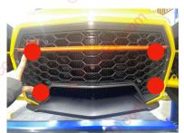
Remove the front grill by removing the 4 bolts marked in red dots above, then pull the grill out towards the front.
