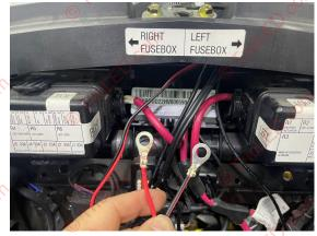
Run power and ground to the battery, connect red to positive terminal and black to ground terminal.
