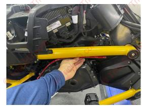
Test fit the LED with the wire towards the front. Clean the surface with the provided alcohol pad and primer wipe prior to installation.
