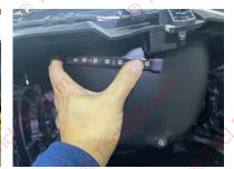
Test fit one of the 14" LED strip, wires toward the rear. Position the LED from front center out to the side and rear.
