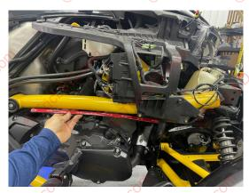
Connect 24" extension wire to LED and run to module. Connect to the 1:2 splitter and into 1 of the open port.
