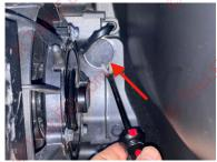
To the rear of the front tub, locate 2 circular plastic cover on the left and right of the tub, and remove.
