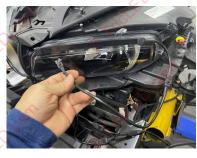
Test fit the 8" LED strip on top of the headlight.
