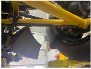
Test fit the LED strip to the rear of the bottom A arm.
