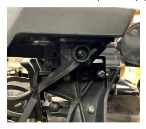
2.-Next take the new screws, washers and nuts and install the armrest back on the new riser mount just like it was mounted to the existing mount. The screw goes in the armrest bracket first then once the screw is in slot add the washer and locknut to the outside. Do not tighten down at this point. Add the other screw as the first. Then before tightening down adjust the armrest forward or backwards to the desired position.
