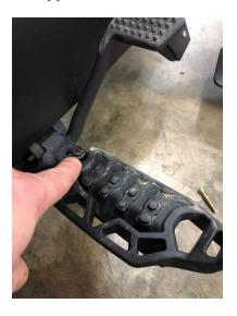
2.- Locate the adapter spacer on the peg support as shown below.
