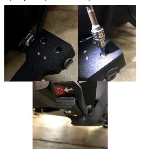
3.- Take the floorboard plate with the letter R facing outwards and the two button heads screws and screw the floorboard plate down. Do the same for the opposite side.
