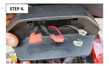
Take the small harness provided in your kit, which has the positive and negative piggyback connectors, and connect the OEM positive and negative female connectors to the male positive and negative connectors of the small harness.
