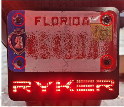
**STEP 8.** Use the remaining 4 screws provided in your kit to attached your license tag using the inner holes predrilled in on your mounting plate.
