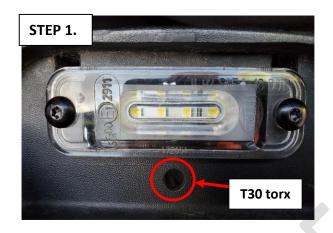
**STEP 1.** Begin by using a T30 torx screwdriver to remove the T30 torx screw located under the lip of the rear fender trim cover.
