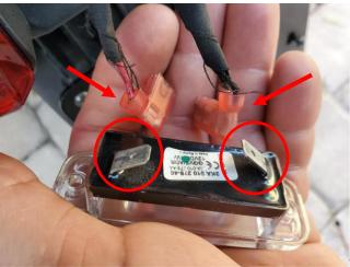
STEP 3, Use a T15 torx screwdriver and remove the 2 torx screws that hold the OEM license plate light in place.
