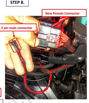
Route the female connector of your new Hazard Light Harness through the opening in the bottom of the cluster support.
