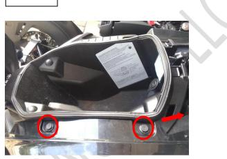
Open the glove box and remove the 3 pushpins from the fairing on the left hand side fairings.
