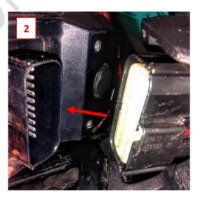
Pull the Multifunctional Gauge away from the cluster support far enough to expose the female connector from the OEM harness.
