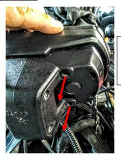
Remove the 4 retaining torx k50 x 16 screws from the back of the Multifunction Gauge utilizing a T20 torx bit.
