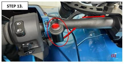
(1) Route the wire coming from the activation button along the back of the handlebar and secure with zip tie.
