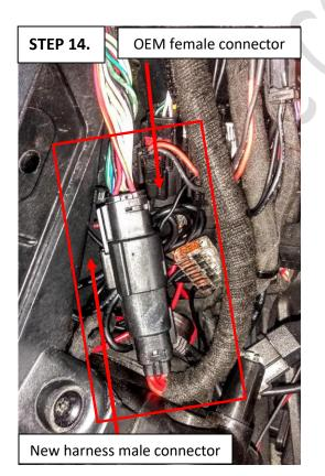
Now to complete the installation of the harness, locate the male connector from your new Hazard Light Harness and connect it to the female connector from the OEM harness.
