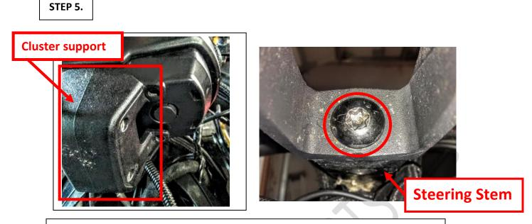
While holding onto the cluster support, take a T40 torx bit and remove the m8 x 25 torx screw that holds the cluster support to the steering stem. Remove OEM steel cable support that holds the cables in place. It will not be reused, use a zip tie to secure cables together at the end of install to neatly retain cables.
