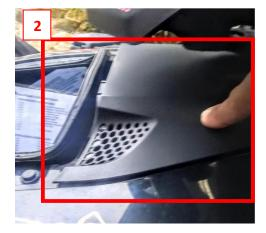
1. Slide the fuel tank flap assembly open and remove the 2 retaining pushpins.
