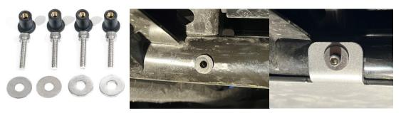
3.- Next take the Skid Plate and locate it under the Ryker with the rear of the skid plate aligned with the two mounting tabs on each side as shown below. Install the suppled screw. Do the same for the opposite side.
