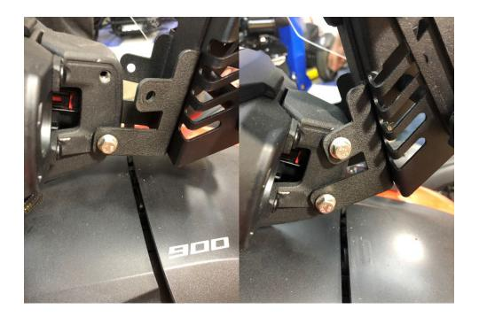
Once installed on your Ryker, adjust the shield up or down to fit your riding needs. When hot outside you can tilt the shield towards you the rider and allow a greater airflow to keep cool. You can adjust the tilt to control the airflow.
