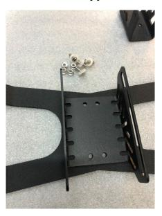
5.-Once the two adjustable mount brackets are secured to the shield mount and the F4 Ryker mount you place them together with the two 3" aluminum spacer between as shown below that allows the mount to slide and tilt.
