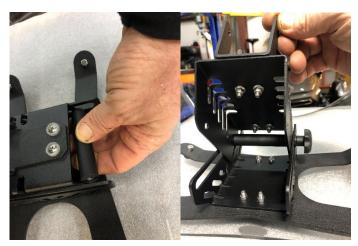
Do this for both 3" spacers using all 4 knobs. You will see that the outer mount bracket has a long slot that when installing the knobs, the spacer is the guide that fits in that slot allowing the two units to slide up and down.
