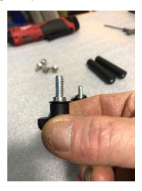
4.- Next take the outer mount of the kit and bolt it to the F4 large windshield mount as shown below. Use the suppled screws, plastic caps, and locknuts in the same way you installed the hardware on the inside mount unit.
