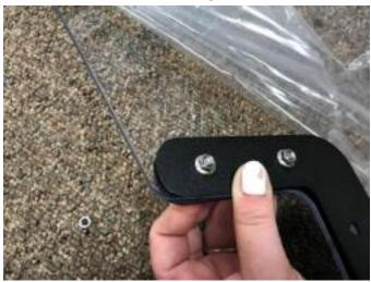
8. To keep the brackets from moving, and to keep the aluminum washers in place use the extra 4mm bolt and nut in the bottom hole. (This will need to be removed before mounting.)
