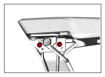
5. Install the assembled armrest using [P6] Torx truss screw M8 X 30 screws and plate [P5].
