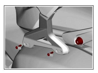
3. When installing with top case, use the washer [P9].
