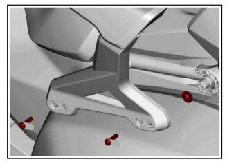
4. Start by pre-assembling the armrest support [P1] and armrest assembly [P3] utilizing the [P7]
