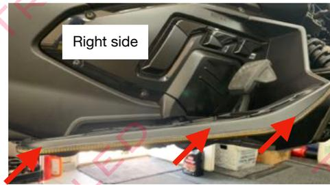
Adhere the LED strip and align with the bottom of the floorboards all the way around. Remember, do not stretch the tubing. The connectors will be towards the rear of the boards on both sides
