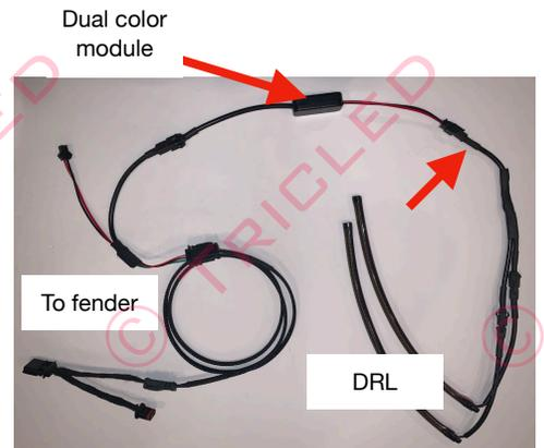
Current setup with Dual color DRL, Insert the 1:2 splitter from floorboards on the red arrow shown above. Then connect your 3' extension and connect to floorboard. Other end of the 1:2 splitter connects back to the DRL
