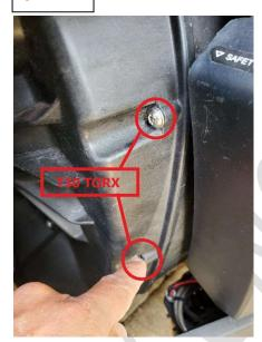
Remove two CVT (Continuously Variable Transmission) cover screws with a T30 torx from the throttle side of your Ryker.
