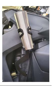
The final step is to tighten the locking nuts installed in STEP 2. Use a 4mm Allen wrench to hold the m6 bolt in place and a 10mm wrench to slowly turn and tighten the locking nuts located on the back of the water bottle bracket until the water bottle holder is secure but be cautious not to **OVERTIGHTEN!**Overtightening may result in cracking the water bottle holder and not covered in your warranty.
