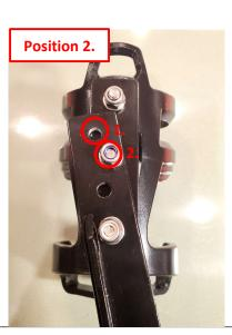
Remove both 6mm locking nuts and washers from the back of the water bottle holder bracket.
