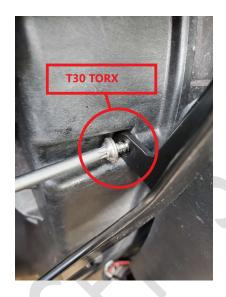
With your T30 torx wrench, use the two CVT (Continuously Variable Transmission) cover screws that you removed in STEP 1 to secure the water bottle bracket to the CVT cover. Slowly tighten the torx screws but be careful not to OVERTIGHTEN.
