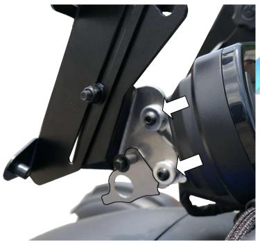
You might have to shift the bracket and posts slightly to get the locking keys to seat completely. MAKE SURE that the keys are fully seated over the bottom posts and down flat against the brackets.
