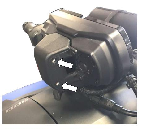
Allen wrench, preferably a ball-end wrench. Do not tighten the screws fully until the brackets have been attached and seated (this will be in Step 2).
