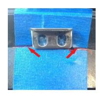
Align the latch catch keeper along the crease in the compartment wall, depicted in the picture in black, and press up against the wall of the compartment to align the pilot holes with in the holes of the latch catch keeper.
