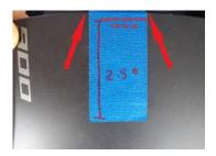
Cut a 2.5" piece of painter tape and center it along the top edge of the trunk lid.
