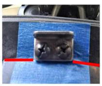
Use the 1/4" screws provided to attach latch catch keeper. Make sure the bottom of the keeper stays aligned with crease in the compartment wall.
