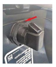
Latch nut must be tightened snug to make sure that the locking washer is properly seated in order to prevent the latch from twisting free.
