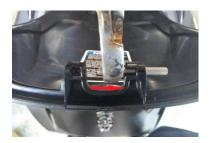
As you face the front of the RYKER, use a pair of pliers to gently twist the push latch catch pin while pulling to the right to remove it.
