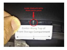
Fold the template along the dotted lines as depicted in red above. Center the template inside the trunk above the USB connector and along the top edge of the storage compartment. Use scotch tape to secure the template.
