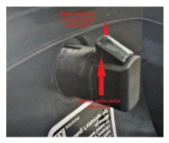
Press down on the latch catch lever while installing the latch through the 1" drilled hole on the trunk lid, making sure that the catch lever is facing up as depicted in the picture above.
