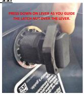
Press down on the latch catch lever and guide the latch nut over it. Make sure it aligns with the latch threads before beginning to hand tighten the latch nut to avoid stripping the threads. Continue to hand tighten until the latch nut is seated firmly against the wall.
