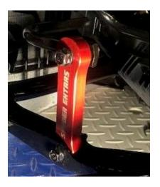
Install the link bottom first. Take the factory bolt and run through the frame channel hole through the spacers / bearing holes. This will push the set alignment screw through the other side.
