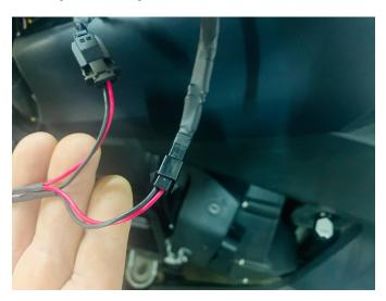
5.- Then tie up the additional wire with supplied wire ties and reinstall the upper front cover.
