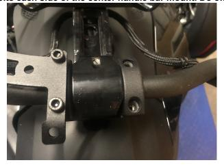
2.-With the supplied new socket head bolts and aluminum spacers, place a spacer in each hole on the handlebar mount. The line up the new docking station arm and place the two new bolts supplied in the holes and tighten down.
