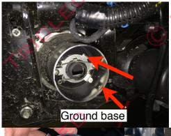
Position the base on the light housing. Make sure it sits flat. There is metal tab on top and bottom and it fits only one way. Once the base sits flat, place the metal clip around the base and re-hook on the metal base. Pull the black wire from the ground base of the light (See red arrow). You will attach this to the black ground on the LED black wire. Connect the yellow positive to the red wire on the LED.
