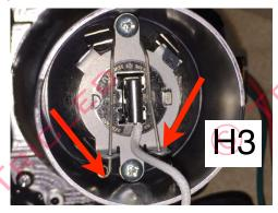
Remove the rubber boot from the back of the outboard lights. Using a long nose plier, undo the metal clip that holds the factory H3 bulb and remove.
