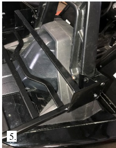
5. install rack with clamp bracket attached
