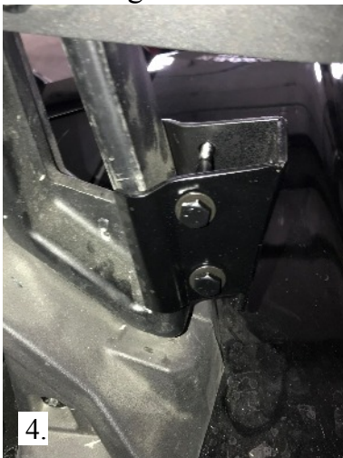
4. right side clamp bracket attached leave bolts loose
