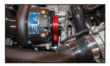
NOTE: Leave these three bolts slightly loose until you install the serpentine belt. Refer to the belt diagram for the belt routing. Once the belt is in place tighten down the three main bracket bolts.
