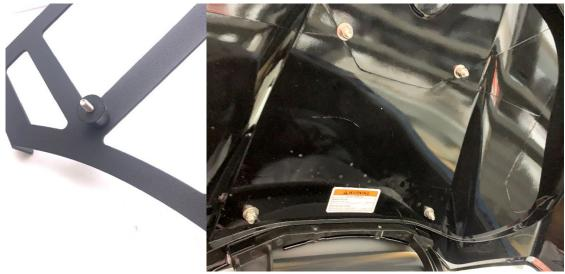
3.-Once completed take the rack and place in position on the trunk. The bolts should drop right in the 4-hole locations. Be sure to use WD-40 or equal lubricant before you put lock nuts on to prevent galling.
