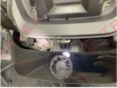
After removing all the bolts and fastener, pull back the rear panel out a couple of inches, locate factory OEM harness behind each taillights. See next picture.
