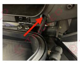
Feed the wire through the inside of saddlebag. Use loom to cover up the wire as it enters the side of the body panel.
