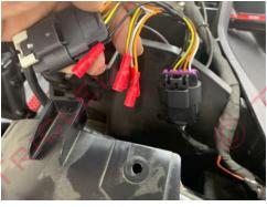
Once the saddle bag wire is up at the top, strip red and black wire ends then crimp male bullet to both.
