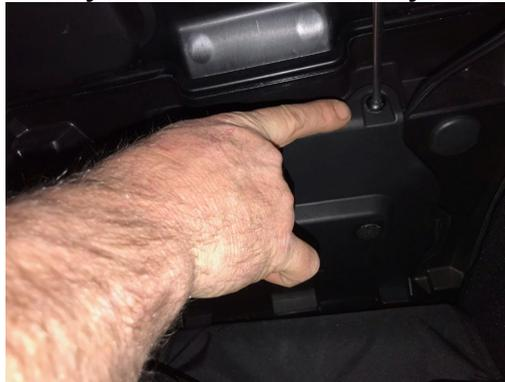
**2.- Remove the access panel under the RT allowing access to the horn location. There will be Push Pins to remove.**
