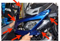
REMOVE THE TWO BLACK PLASTIC COVER UNDER FRONT TRUNK AND UNSCREW AND REMOVE FRONT FASCIA
