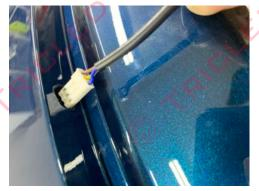
Remove masking tape after drilling. Clean surface with alcohol pad and let dry. Apply primer to surface and let dry. Feed the wire through and pull wire out to the side of metal arm bracket.
