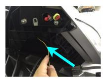
Run the black wire behind this opening and pull it out of the opening where the OEM harness exits. Peel back the OEM harness and use the T-Tap on the positive colored wire. Crimp the black wire with the male spade and insert into T-Tap.
