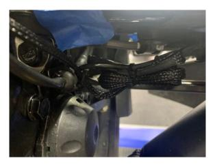
If you are not installing any additional lighting, loop the extension, cover the connector with electrical tape and zip tie under front A arms for future use.
