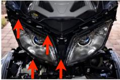
LODSEN UP ALL 4 BOLTS FROM THE HEADLIGHT HOUSING AND PULL OUT SLIGHTLY AND REACH IN AND PULL OUT THE TURN SIGNAL HARNESS FROM BEHIND THE HEADLIGHT. USE THE SUPPLIED T-TAP AND TAP THE POSITIVE LINE ON THE MIRROR AND CONNECT AN EXTENSION WIRE TO THE WHITE BLINKER MODULE AND CONNECT. REPEAT FOR OPPOSITE SIDE.
