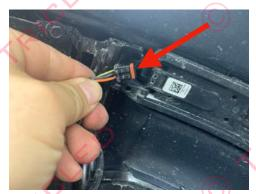
Remove harness from the front LED light. Push center clip and pull back to remove.
