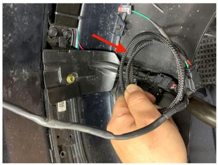
3' extension will run out of the fender to connect any of our single/dual color lighting kit, such as DRL on A-arms or skid plate with LED.
