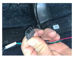
If installing optional kit 1:2 splitter harness for the DRL, connect 1:2 splitter into fender harness. Connect one side of the splitter to 3' extension. Connect the other open side of 1:2 splitter to factory OEM wire.
