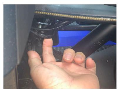
Run the extension out of the fender and across the bottom of the A arm to reach the DRL module towards the center of the bike. Zip tie all loose wires.
