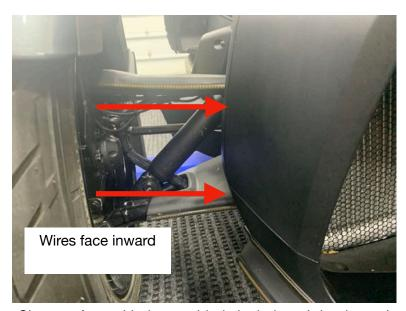
Clean surface with the provided alcohol swab let dry and apply primer. Install LED with wires facing inwards towards center of bike.
