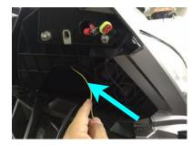
Run the black wire behind this opening and pull it out of the opening where the OEM harness exits. Peel back the OEM harness and use the T-Tap on the positive colored wire. Crimp the black wire with the male spade and insert into T-Tap.
