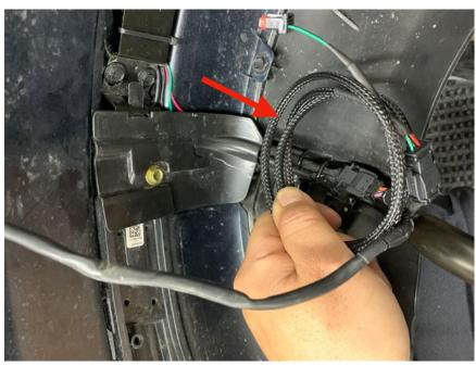
3' extension will run out of the fender to connect any of our single/dual color lighting kit, such as DRL on A-arms or skid plate with LED.
