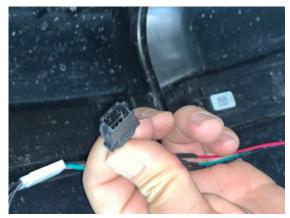
Install1:2 splitter harness to the front fender LED light. Connect one side of the splitter to 3' extension. Connect the other open side of 1:2 splitter to factory OEM wire.
