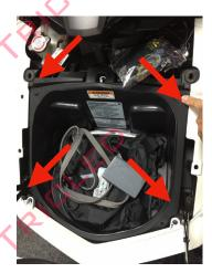
Remove the 4 push pins on the front trunk tub and remove to expose the battery.
