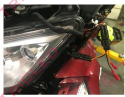
For the 2019 model, there is no longer a harness up front and power will now be taken from this 2 pin OEM harness behind the factory headlight. Remove fairing and headlight on one side only.
