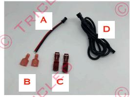
Use the T-Tap(C) and crimp the factory customer accessory harness. Crimp spade(B) to the (A) harness ends. Connect (A) to (D) harness. Ue Di-Electric grease on all connectors to prevent corrosion. Connect (D) harness and route it to the bottom and connect it to the Skidplate LED.
