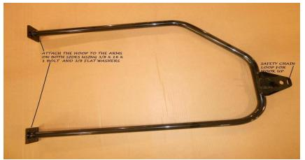
Leave bolts loose for now. Next, place strut bushings into the tube on the frame above the fuel tank. note:\*\*some de-burring may be required inside the tube.
