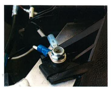
13. If you have a pre-2020 model, run the red power wire as shown down to the battery. Cover the wire with one of the shorter lengths of split loom (not shown in pic). Skip to step #19.
