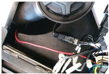
14. For 2020+ models, run the red wire from the isolator along side the yellow wire over to the right side of the Slingshot. Cover them both with the supplied shorter lengths of split loom.
