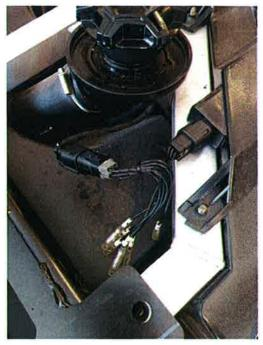
3. Connect the yellow jumper wire to the wire marked "3" on the right side SUB-HARNESS. Please note that the remaining 5 wires on the right taillight will remain unused.
