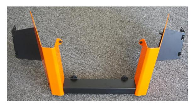
**Step 3 – Hardware C:** The left and right Bumpers get connected together by the Crossbar as shown below. Screws go through the crossbar into the bumpers, then put flat washers and nylock nuts on the insides of the bumper and snug them but don't fully tighten. Make sure they are even with each other and at that point tighten all six screws and nuts fully. This now becomes the **Bumper Assembly.**
