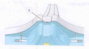
3. Remove the fastener (8) under the center trim piece on the back of the rear body panel.
