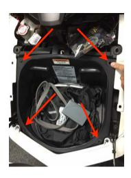
Open front trunk, remove the top service cover by pulling up on the rubber grommet. Remove the (4) push pins on each corner of the trunk tub, pull up and remove the trunk.
