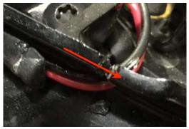
On the left side of the trunk lip there is a plastic holder with a hole. Using a side cutter cut the top section to slot (cut straight line down to the hole opening). You can slide the wire through the top as shown above.
