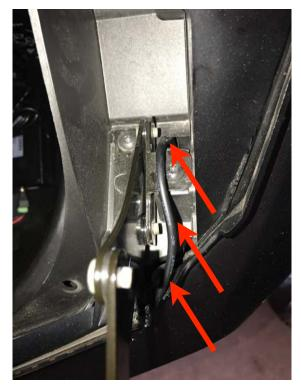
Run the Knight rider LED through the outside of the hinge and insert into hole opening by the hinge. Pull the wire out from the bottom side.
