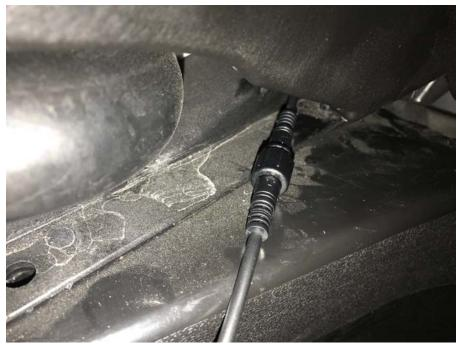
Once the wire is pulled out from the bottom side, put some Di-Electric grease on the inside connector. Line up the pins and insert the module side into the knight rider LED wire. Route the wire along the edge and zip tie it on the back wall where all the wiring harness is located.
