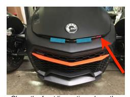
Clean the front lip section where the LED will be adhered to. Apply multiple coats of 3M primer and let dry. Use masking tape and hold the center section while the adhesive cures against the front hood.
