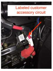
Two ways you can connect the knight rider LED. First option is direct to the battery and the other is through the ACC wire which will only be on when the bike is running. For ACC wiring , look on the right of the battery box and locate the factory harness labeled "customer accessory circuit". Peel back the protective covering and it will reveal 2 loose open wire. Connect the knight rider LED here.
